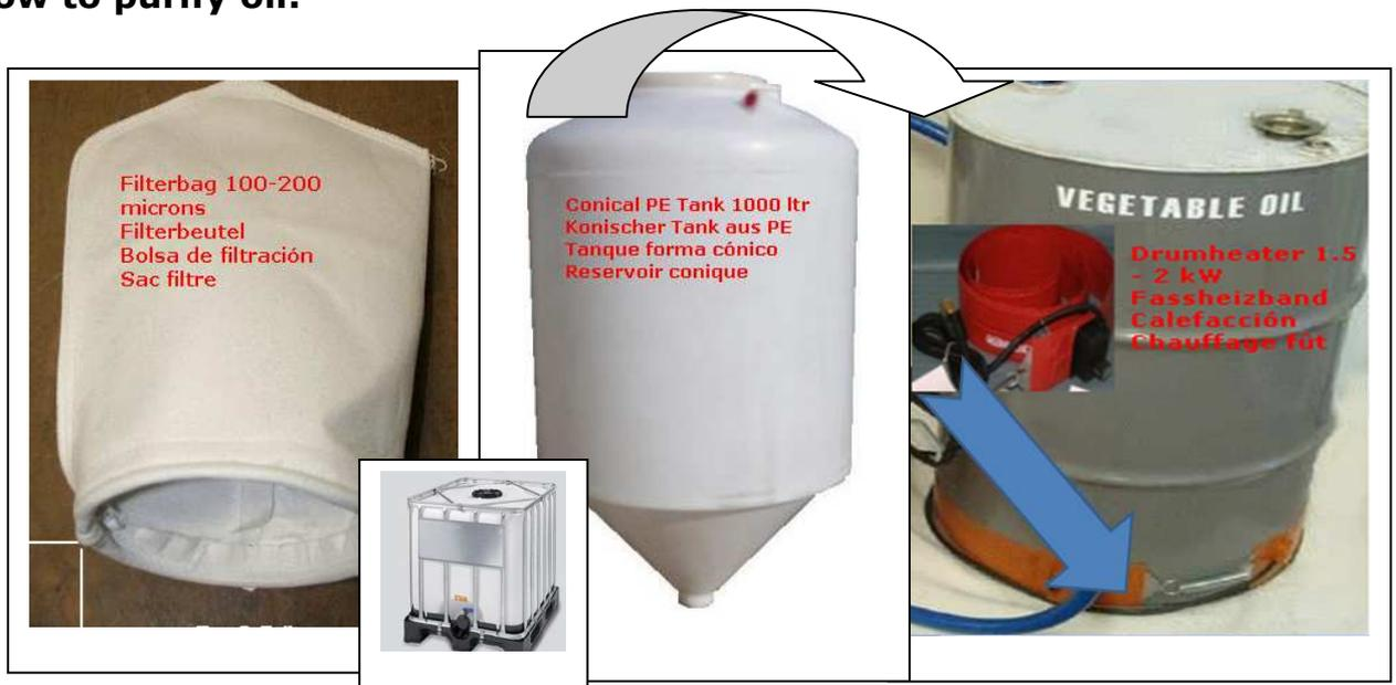
1. Pour the oil into a preferably conical HDPE tank (reactor tank) in a room at 20°C (do not heat the tank as this causes convection and mixing currents) allow the oil to settle over a few days. You may also use other tanks with a flat bottom. Use either a filter bag 200 $\mu$  or a rough 500 $\mu$  sieve – in the second case you can use a suction filter
