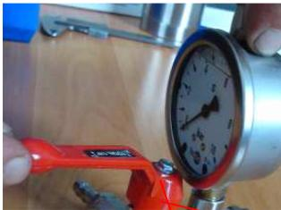
By opening and closing the ball valve(yellow or red lever in illustrations) the return to the container(barrel) will take more or less flow - as a results the pressure entering the centrifuge can gradually be adjusted to a Maximum of 7 bar, the rotor starts to turn at appr.2 bar **Please also read last pages for safety**
